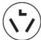
3-wire receptacle (10-30 R)
