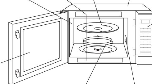
**Roller Ring and oven cavity floor:**
