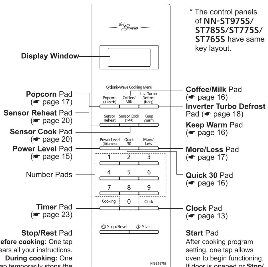
\* The control panels of NN-ST975S/ST785S/ST775S/ST765S have same key layout.
