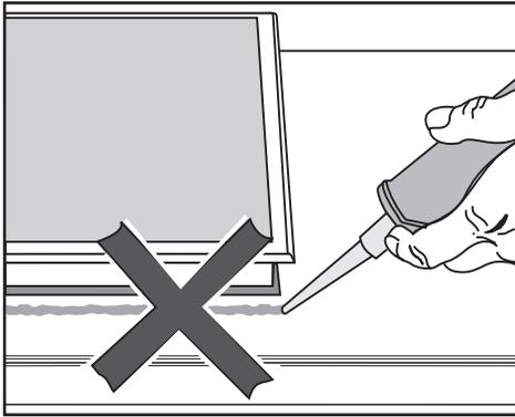
NEVER use sealing unless it is explicitly called for in the instructions. The sealing strip under the edge of the upper part of the appliance provides a sufficient seal against the countertop.
