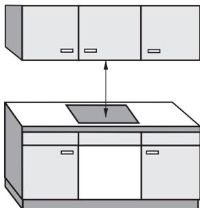
If there are various appliances with different recommended clearance distances beneath the exhaust hood, e. g., a gas stovetop and an electric cooktop, always choose the greatest distance.
