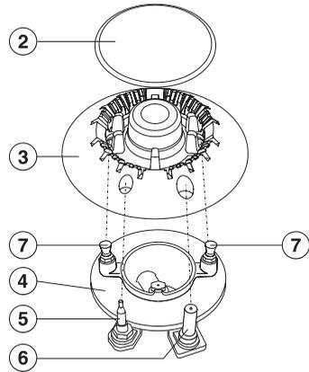
■ Arrange the burner head ② on the lower part (base) of the burner ④ in such a way that the thermocouple ⑤ the ignition electrode ⑥ and the retaining pins ⑦ align through the holes in the burner head.
