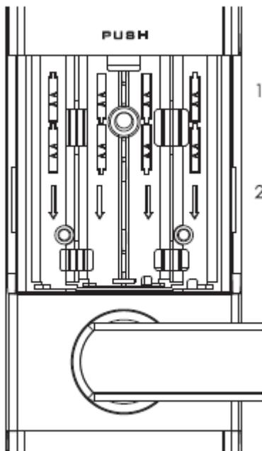
1. In the battery box you can put 8 AA 1.5V Alkaline batteries maximum. It can be used for over one year(10 times per day). Battery life is relative to user's using habits, using environment, optional function and so on.
