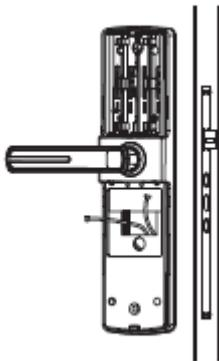
4.8 Fasten 4 mounting screws. Insert the connecting cable and lock case cable into the ports on inside escutcheon.
