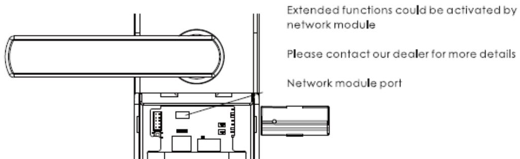
Extended functions could be activated by network module.
