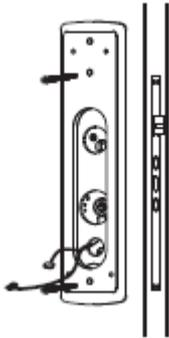
4.7 Put the shaft spring and shaft into the hole of inside escutcheon. Insert the shaft of inside escutcheon into the hole on the lock case and keep inside escutcheon close to the door.
