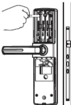
4.9 Install batteries, battery box cover and inside escutcheon bottom cover. Installation finished.
