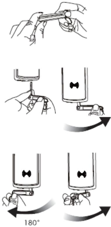
Insert the mechanical key into the key hole and turn the key, then you can push handle to open the door.
