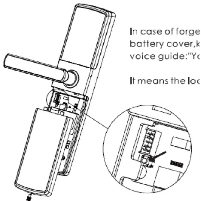
In case of forgetting master PIN code, you can remove the battery cover, keep pressing the reset button for over 5 seconds. Voice guide: Your lock has restored to factory settings.
