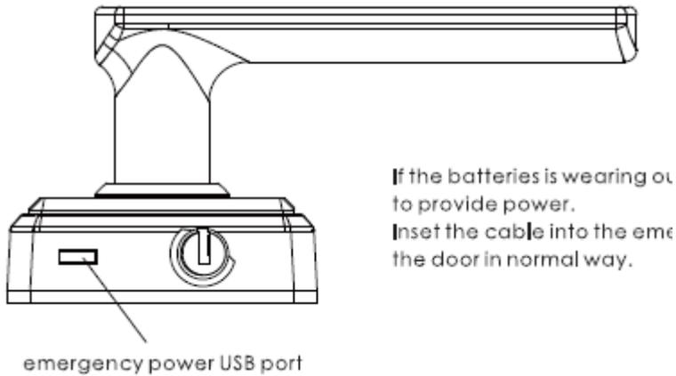
If the batteries are wearing out, you can connect micro-USB 5V to provide power.
