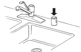
The drain air gap is usually located on top of the sink or countertop near the dishwasher.
