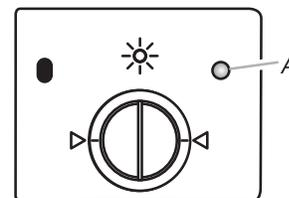
**NOTE:** For most water conditions, the factory setting of 2 will give good results. If you have hard water or notice rings or spots, try a higher setting. Turn the arrow adjuster inside the dispenser by either using your fingers or inserting a flat-blade screwdriver into the center of the arrow and turning.
