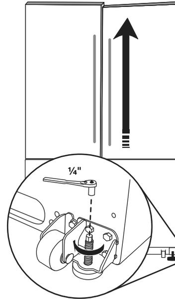
6. Make sure the refrigerator is steady. If the refrigerator seems unsteady or rolls forward when the door or drawer is opened adjust the leveling screws. Using a 1/4" hex driver, turn the leveling screw on each side clockwise until the rollers are up and the leveling feet are firmly against the floor.
