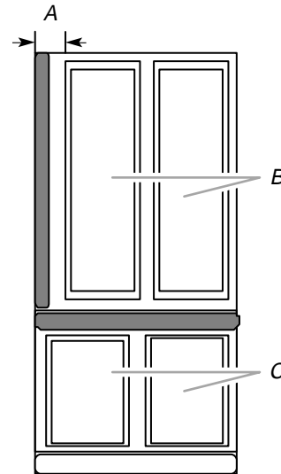
A. 2\frac{1}{2} " (6.35 cm) Clearance B. Raised decorator panel C. Raised drawer panel
