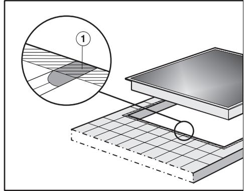
The grouting ① and shaded area under the cooktop frame must be flat and even, so that the frame will lie evenly and the sealing strip under the edge of the upper part of the appliance can provide an adequate seal against the countertop.
