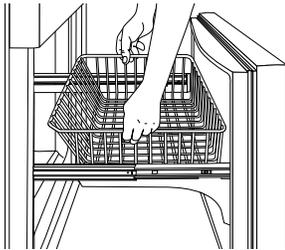
5. Remove the basket cradles from the drawer rails. Push the snap attachments inward away from the drawer rails to unlatch the basket cradles. Lift the basket cradles off of the drawer rails.
