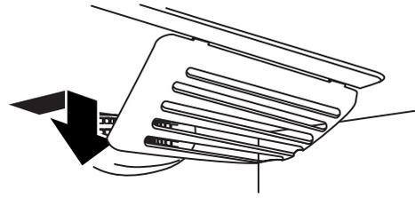
3. Remove the cover and replace the burned-out bulb with an appliance bulb no greater than 40 watts.
