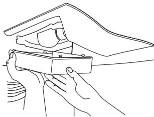
3. Replace burned-out bulb(s) with appliance light bulb(s) no greater than 40 watts.
