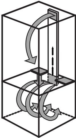
Do not block any airflow vents. If the vents are blocked, airflow will be obstructed and temperature and moisture problems may occur.
