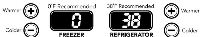
**IMPORTANT:** When the power is on, the temperature display shows the actual temperature of the compartment.
