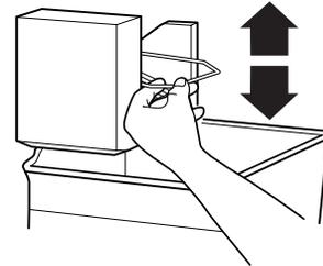
2. Install the interior water filter. The interior water filter mounting bracket is located on the left side wall of the refrigerator compartment.
